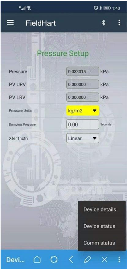
The user shall click the button in the lower right corner to view "Device Information", "Device Status" and "Communication Status".
